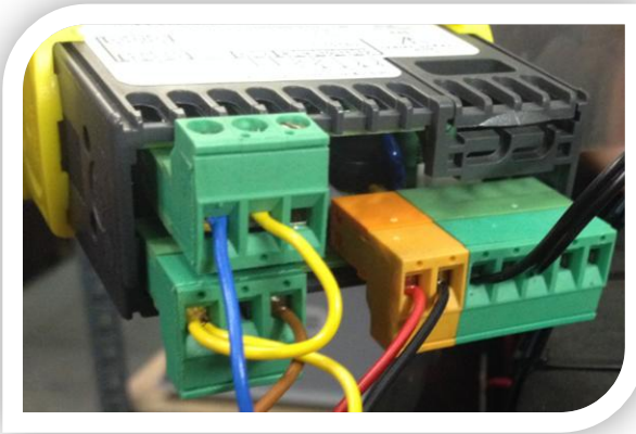
Connecting the IR33W7LR20 (advanced version)
